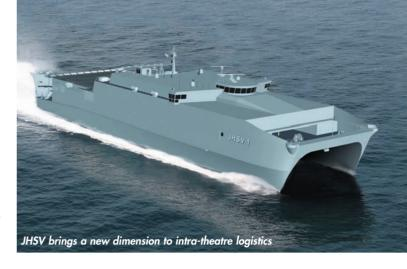
capabilities to a high-speed commercial ferry - and hence adopting commercial international survivability standards - but modified to incorporate a flight deck and aviation facilities, vehicle deck offload ramp and appropriate firefighting, C4I and force protection facilities. An initial buy of 10 JHSVs has been approved - split equally between the Army and Navy - with prospects for follow-on orders.
